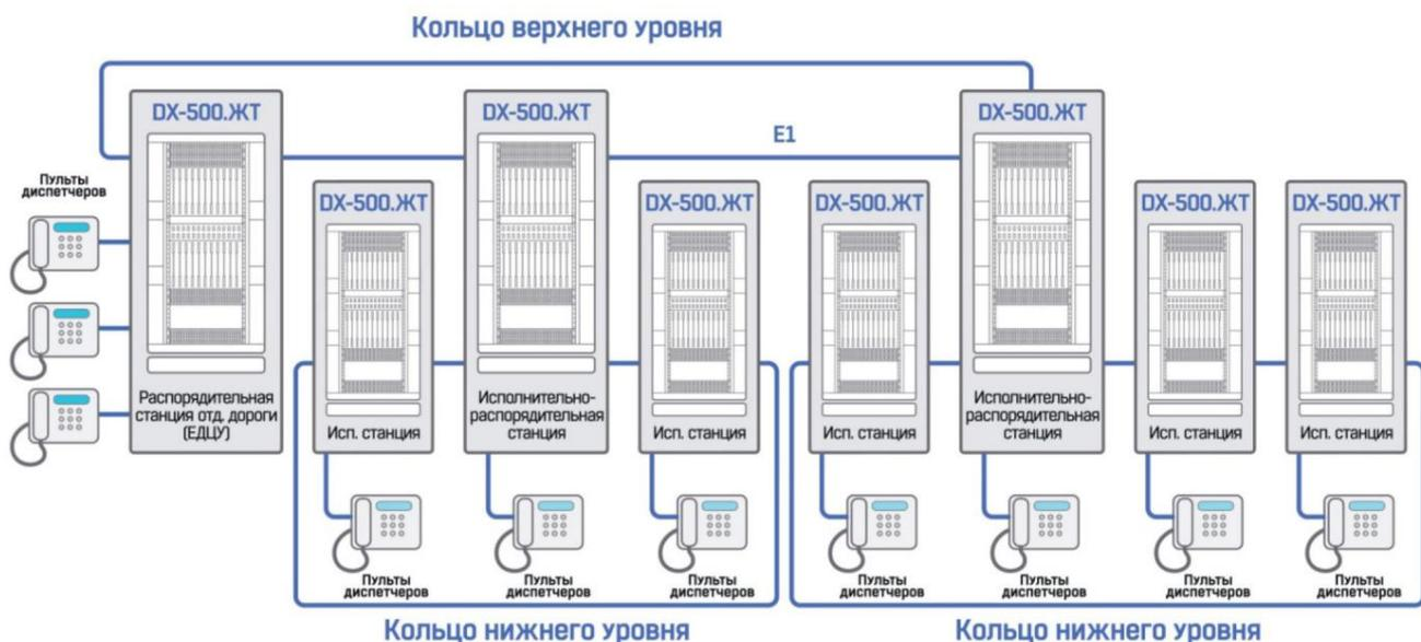
The OTS network based on MiniCom DX-500.ZhT stations is built on the principle of rings, which makes it possible to achieve high reliability of the communication system in the event of a break in the linear path. The equipment of executive station sections (up to 30 stations) is connected by a lower-level ring.
